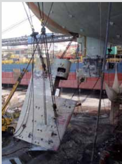
▲ Rudder blade shifted out
