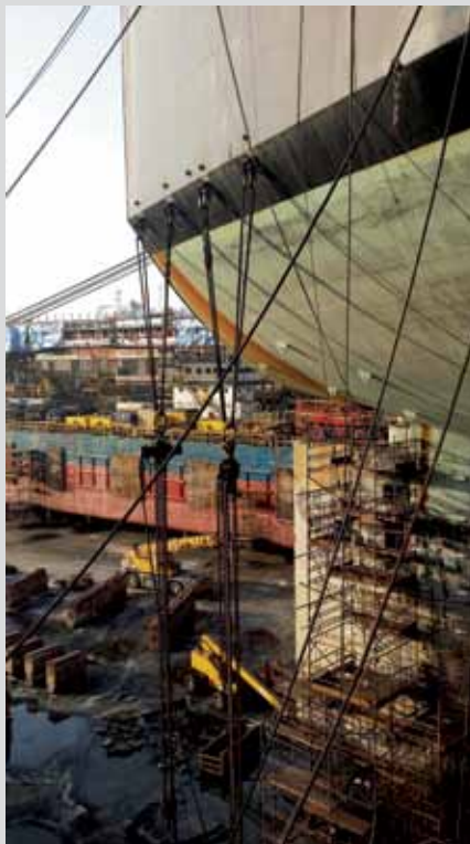
▲ 4 x 100 ton chain block fitted on padeyes for removal of rudder blade.
