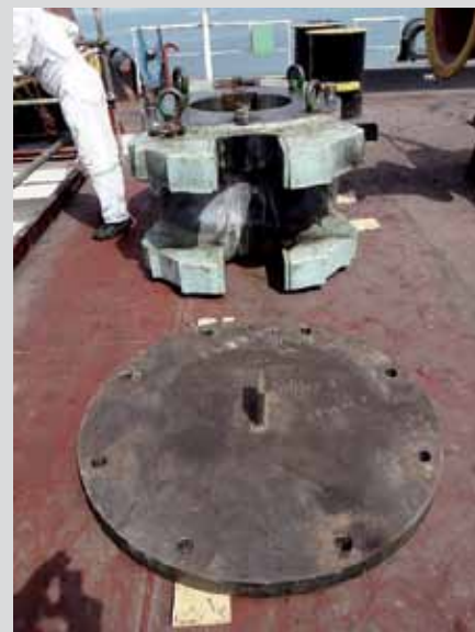
▲ Rudder tiller on the poop deck
